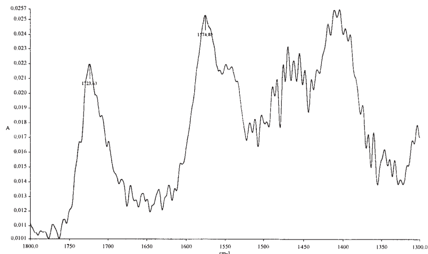
Figure 10 Differential ATR-FTIR spectrum of BTCA/ \beta -CD-finished cotton (100 g/L \beta -CD, 6 g/L BTCA, and 6 g/L SHPI in the finishing bath) rinsed in cold water and washed at 60°C for 30 min after an alkaline solution posttreatment (the spectrum of cotton was subtracted).
