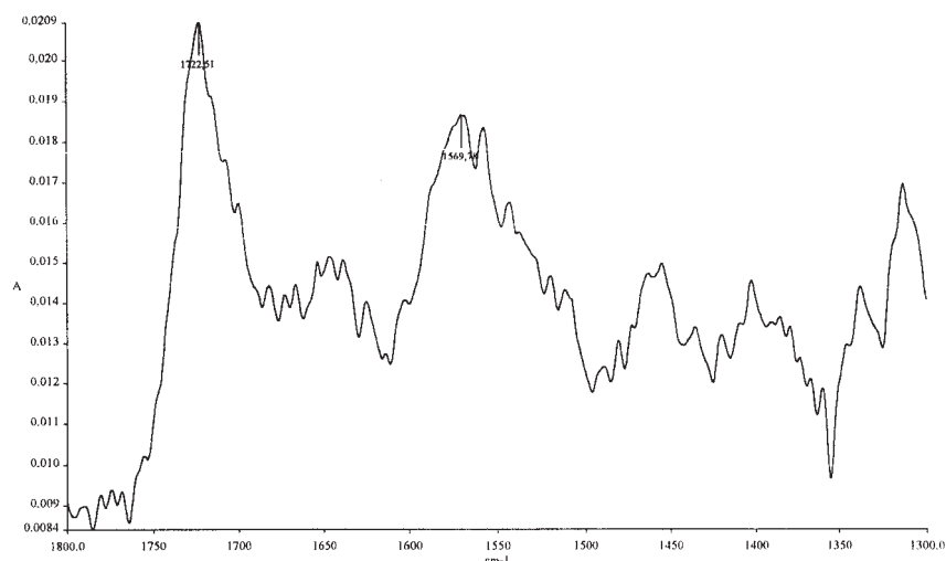
Figure 11 Differential ATR-FTIR spectrum of BTCA/ \beta -CD-treated cotton (curing was carried out at 200°C without the addition of SHPI at 200°C) rinsed in cold water and washed at 60°C for 30 min after an alkaline solution posttreatment (the spectrum of cotton was subtracted).
