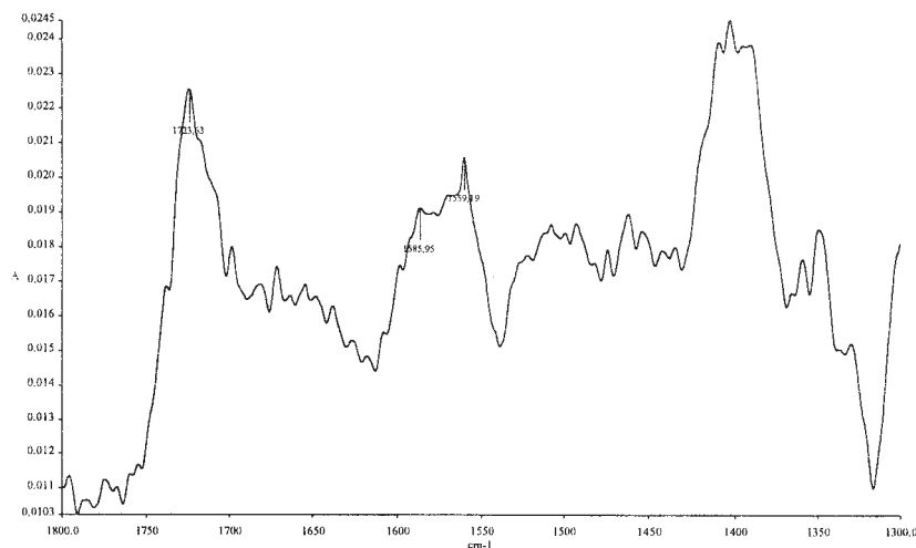
Figure 9 Differential ATR-FTIR spectrum of BTCA/ \beta -CD-finished cotton (100 g/L \beta -CD, 6 g/L BTCA, and 6 g/L SHPI in the finishing bath) rinsed in cold water after an alkaline solution posttreatment (the spectrum of cotton was subtracted).
